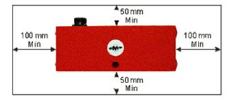
To avoid interference between two Transceivers, there must be a minimum space between them.
